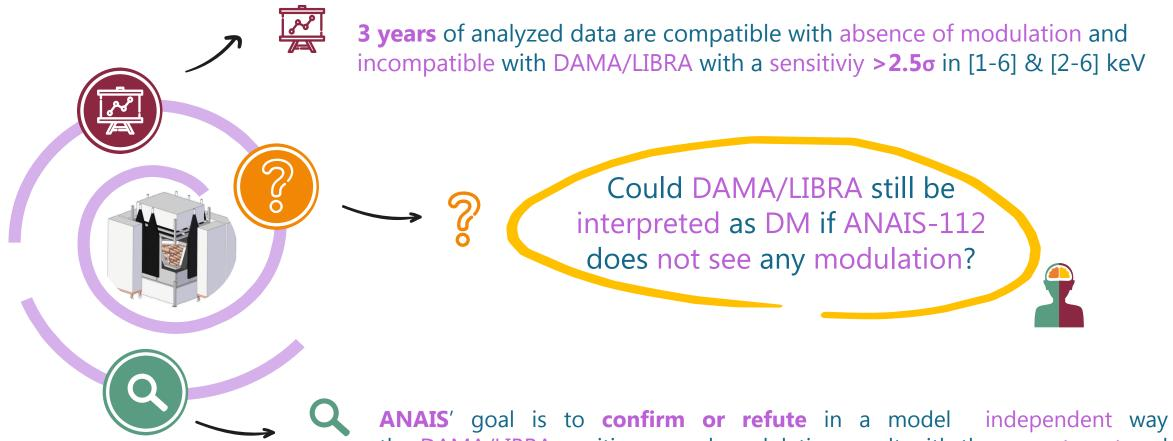
ANAIS' goal is to confirm or refute in a model independent way the DAMA/LIBRA positive annual modulation result with the same target and technique (but different experimental approach and environmental conditions) at the Canfranc Underground Laboratory (@Spain) with 112.5 kg of NaI(Tl)
